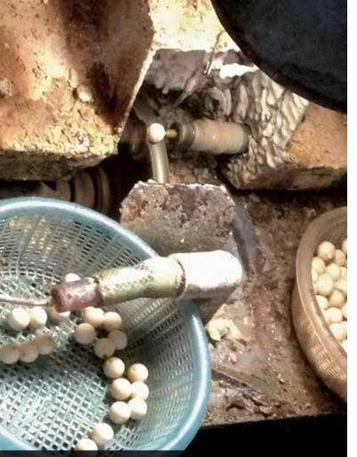
This machine drills holes through larger beads with water trickling down the trough to settle the ivory dust.
