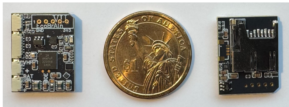
Figure 1. Sensor node hardware. Top side (left board): Apollo 4 Plus MCU in the center, high-efficiency regulators along the bottom, external connectors (power, VHF, programmer, and microphone interfaces) on the left, plus an integration header at the top. Bottom side (right board): MicroSD card slot and low-power components in a low-noise area.
